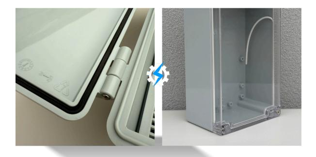
Black sealing gaskets are made by machine injection molding, resulting in no gaps, a tight fit, and integration with the lid, making them impossible to remove. To ensure the gasket is more secure, the waterproof box should be assembled only after the injected material has cooled.
